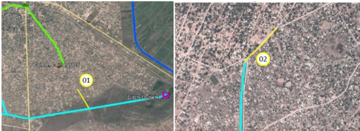
Figure 4: Conceptual design of new drainage channel in neighbourhood 4 (right) and 5 (left)
