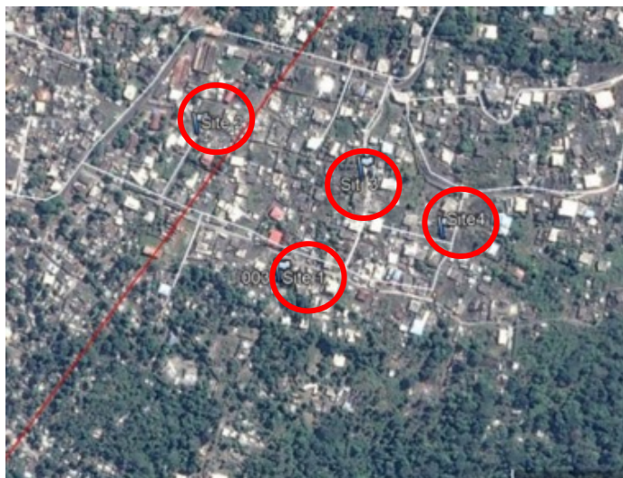
Figure 4: Identified locations for installing the 4 community-based rainwater harvesting systems in La Coulée
