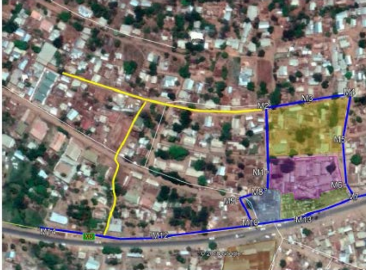
Figure 6: Proposed locations and conceptual design of drainage intervention in Chinamwali
