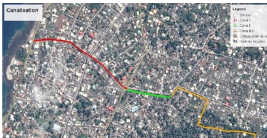
Figure 1: proposed drainage channels for La Coulée neighbourhood
