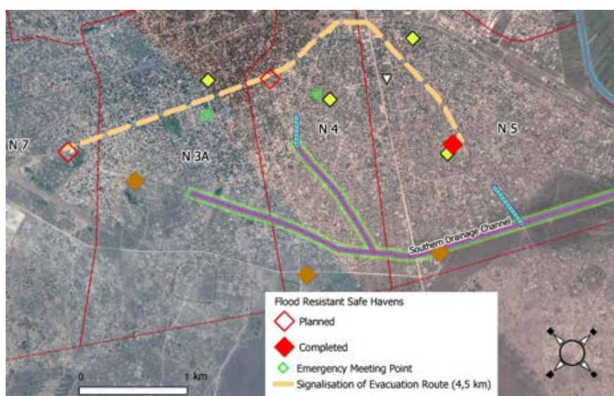
Figure 5: Location of the 3 safe-havens in Chokwe, one already completed and two to be built; an evacuation route links the 3 structures
